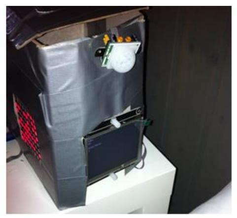
Figure 1: SleepCompete prototype. The LED Matrix displays the score visualization
