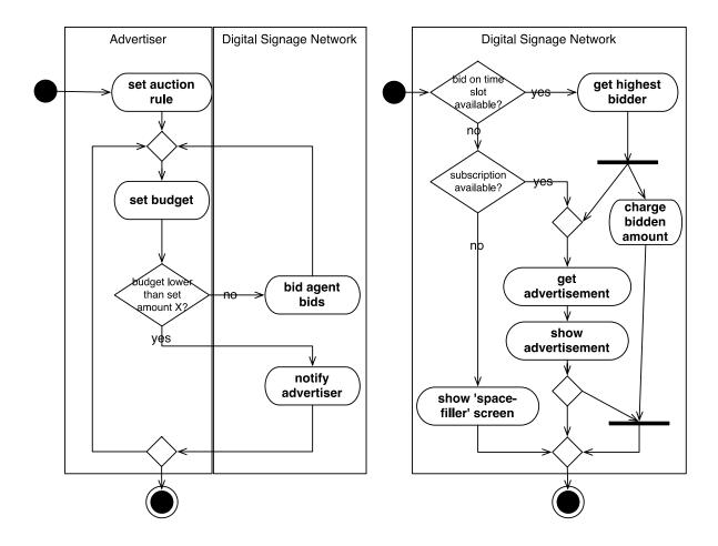
Figure 3. UML activity diagram for an exemplary rule set and backend services
